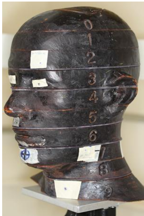
Figure 5: RANDO® phantom with PMMA templates in place
