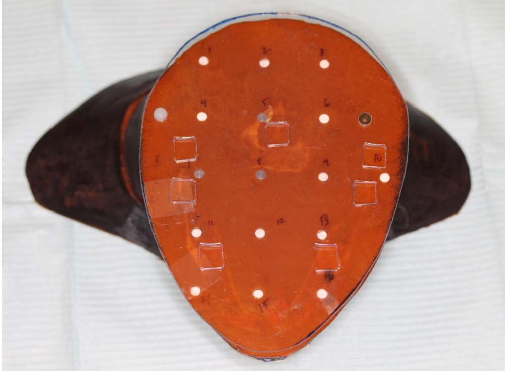
Figure 4: PMMA template for OSLD placement
